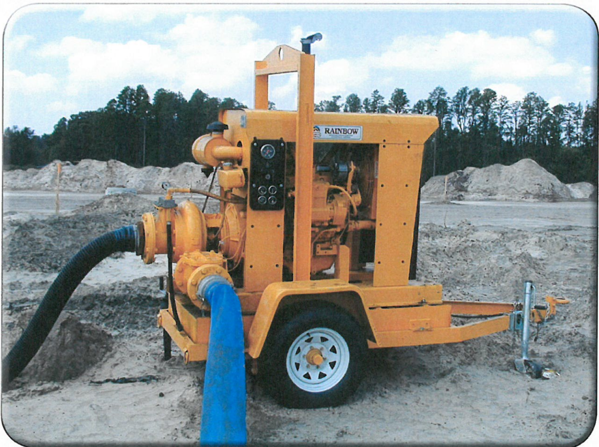
Dewatering Pump (Diesel) Capacity: 2>> - 4>> - 6>>
